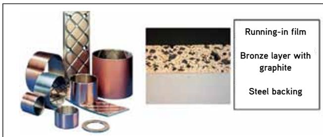
Image 4 (deva-bm + micrograph) A thin-walled bi-metal material comprising a steel backing (seawater resistant) with a sliding layer of deva.metall®. The latter is either graphite or PTFE.
